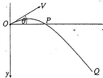
A projectile is fired from 0 with speed  $V \text{ ms}^{-1}$  at an angle of elevation of  $\theta$  to the horizontal. After  $t$  seconds, its horizontal and vertical displacements from 0 as shown are  $x$  m and  $y$  m.
